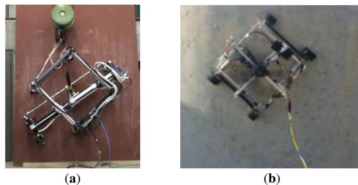
**Figure 3.** Wall-climbing robots.; (a) sandblasting robot [Reproduced from [51] with permission from Richard J. Duro]; (b) EJBOT [Reproduced from [52] with permission from Mohamed Gouda Alkala].
