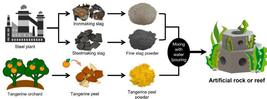
Fig. 12. The flow chart of processing wastes from steel plant and tangerine orchard into artificial rock or reef for seaweeds cultivation.
